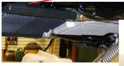
LET THE ELEMENT HANG AND DRILL THROUGH FRAME AT MARK. USE A 17/64" OR 1/4" DRILL BIT. (17/64" FOR MORE WIGGLE ROOM).
