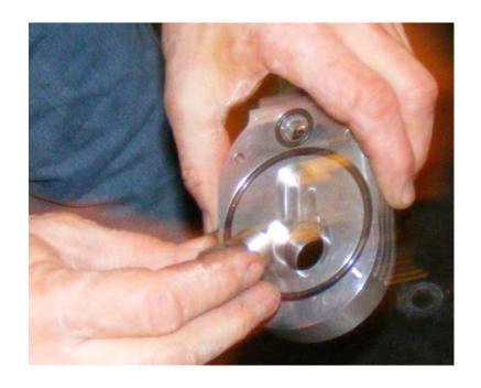
INSERT THE OIL BUD NUT INTO THE INNER ADAPTER HALF.
