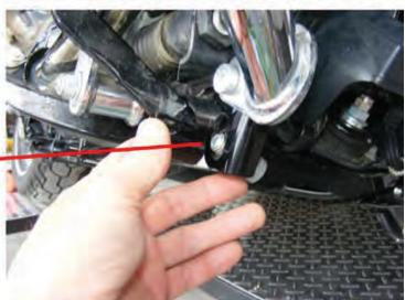
Screw hose to Oil Bud<sup>TM</sup> cooler - hand tighten fitting to cooler
