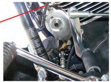
Remove right side floor board support allen bolt.
