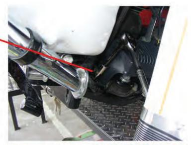
Take nut off front motor mount bolt. Lift regulator up and turn around. Leave large area washer on bottom. Install supplied self locking jam nut over top of existing factory nut.
