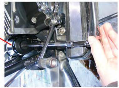
Remove Oil Filter Threaded Bolt that holds filter from engine.
