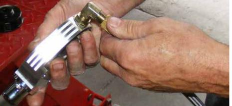
INSTALL THE 'LONG' HOSE ON JIC FITTING USE THE 9/16" WRENCH TO HOLD THE JIC TIGHTEN THE HOSE FITTING COMPLETELY WITH THE 11/16" WRENCH
