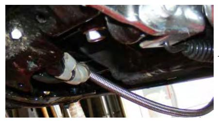
PUSH UP THE SHEATHED WIRING TO MAKE ROOM FOR THE FRONT COOLING ELEMENT THAT YOU WILL PREPARE ON THE NEXT STEP.
