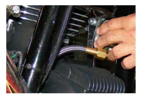
WHEN YOU ARE SURE YOU HAVE THE O-RING IN PLACE' LINE UP THE ADAPTER BETWEEN FRAME AND O2 SENSOR. LINE UP THE THREAD BOLT TIGHTEN 'BARELY SUNG'.
