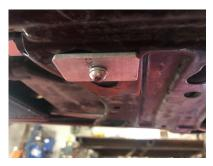
PUSH ELEMENT INTO PLACE. WARNING- NOTE: THERE MUST BE ROOM BETWEEN THE MIDDLE COOLER ELEMENT AND THE ENGINE CRANKCASE. THE ENGINE WILL SHAKE BECAUSE OF A RUBBER MOUNTING AND CANNOT BE ALLOWED TO RUB ON COOLER ELEMENT.
