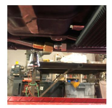
FINISH COOLER ELEMENT HOOK-UP. DO NOT TIGHTEN YET. INSTALL RETAINER CLAMPS TO BRACE AND REAR ELEMENT TUBE, SNUG ONLY. NOW HOOK UP HOSE TO REAR ELEMENT.
