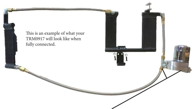
Attach hose to inside half of adaptor as instructed in "STEP 3". Continue installation and feeding of hose as show up through "STEP 7". Follow ALTERNATE STEPS based on model as stated "7a for 2009 and 7b 2010 up".
