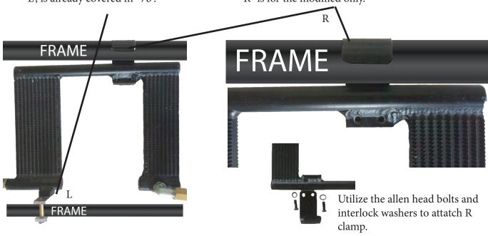
Adjust front element until it has sufficient clearances and does not rub against surrounding. Tighten brackets to keep support intact.
