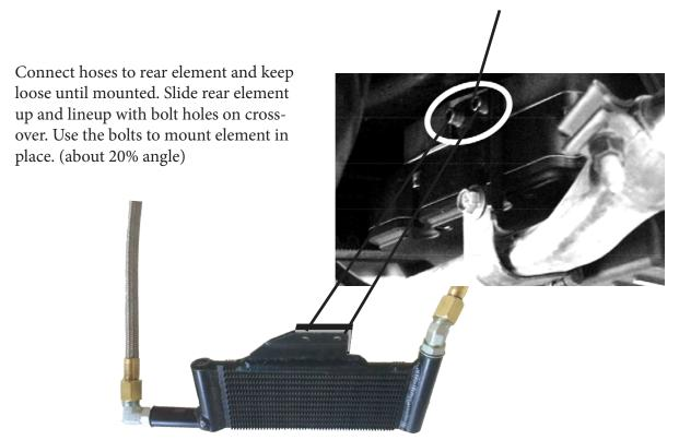
\* Note that step "7c" is not in this application. The rear element clamp will not be neccesary.
