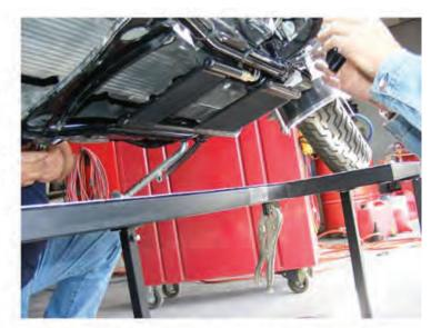
Re - install allen bolt through the slot in the cooler through the frame bracket to floor board then tighten.
