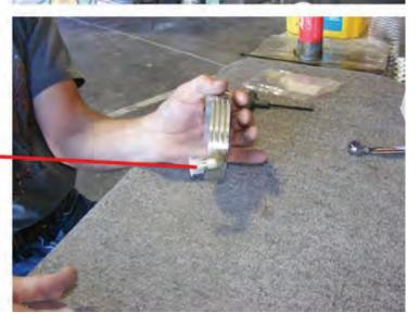
Take inner half of the provided adapter (has the chrome top piece) and install longer hose on adapter and hand tighten for now.
