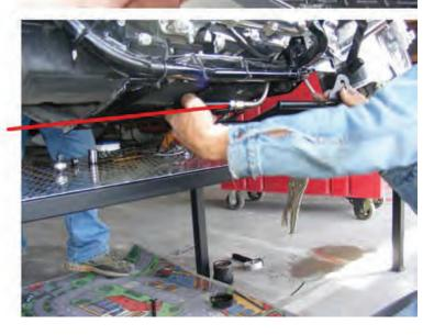
Manipulate brackets into frame rails on left side of frame. Be careful not to put undo stress on hose assembly!
