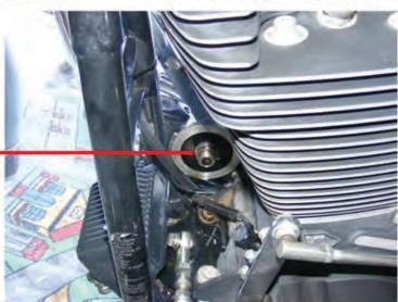
Put grease on O-Ring fitting on the inner adapter half (has the chrome cap)
