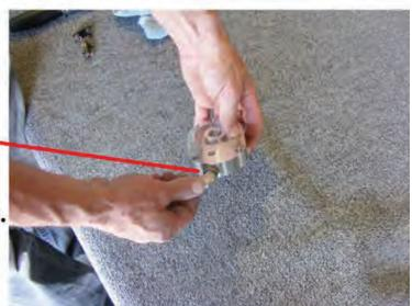
Put grease on small O-Ring and larger O-Ring. Match adapter halves, then install bottom shorter allen screws 'loosely.'
