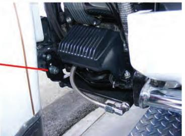
Once proper angle of fitting is attained, Tighten O-Ring lock nut fitting.
