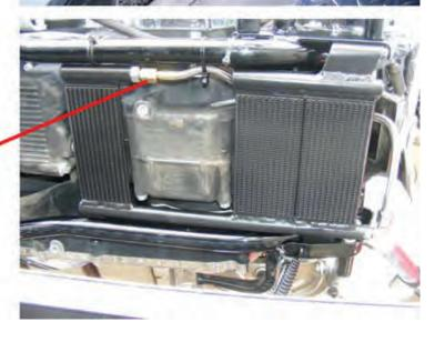
Take outer half of adapter & lightly grease threads of fitting. Then install O-Ring fitting to the adapter.
